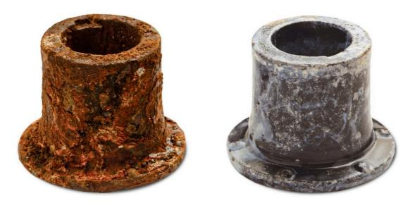
Two collars showing the difference in corrosion after three weeks of salt spray on coated and uncoated surfaces.
